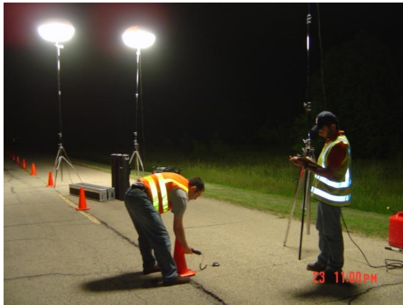
Figure 4.20 Horizontal Illuminance Measurements
