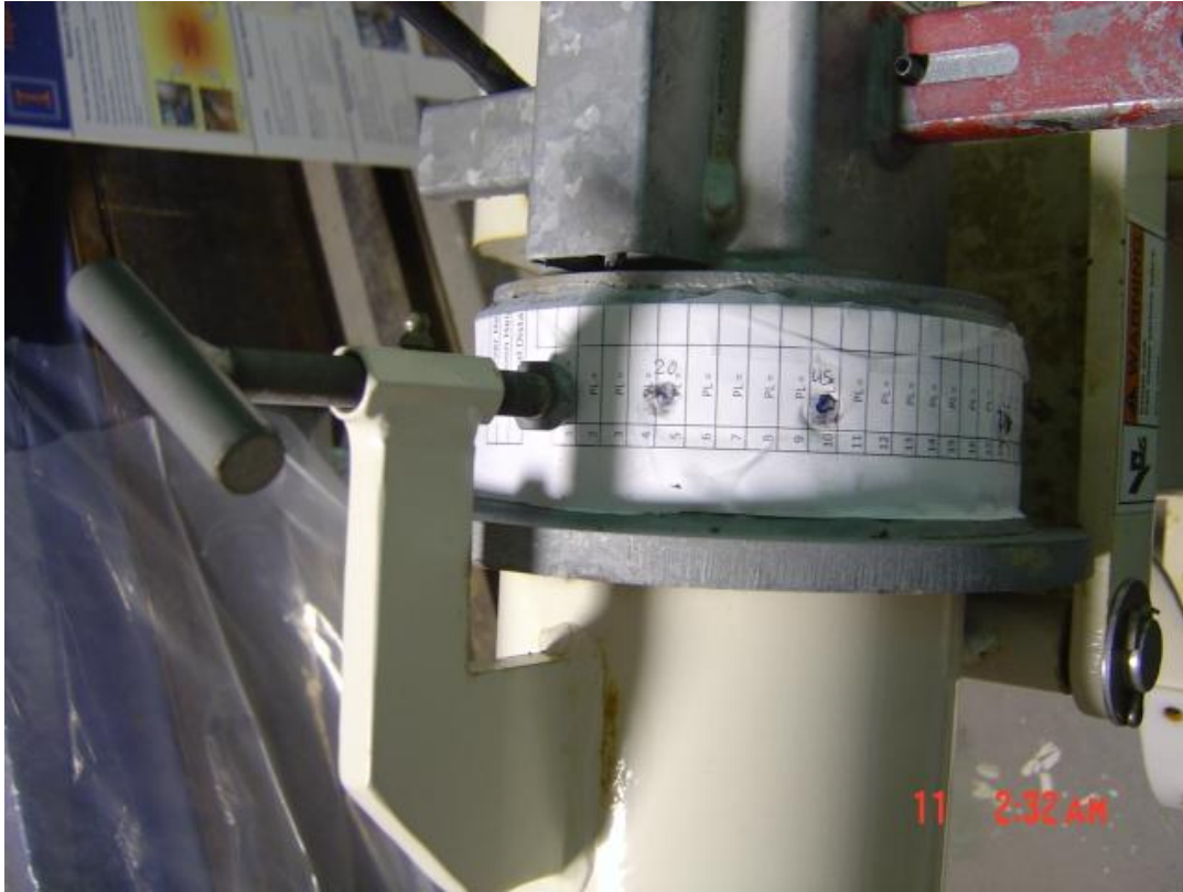
Figure 4.12 Angle Locator Used to Measure Rotation Angles
